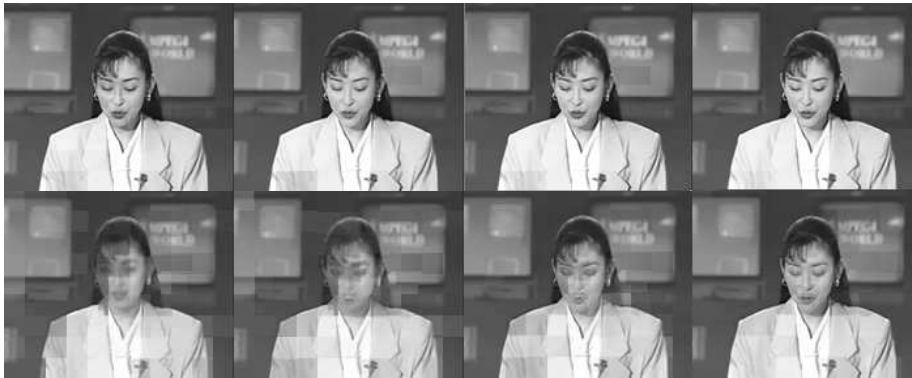
Figure 4.8: Subjective video quality of the 45 th "Akiyo" video sequence frame using SECCC Scheme (top) and Benchmarker scheme (bottom) summarised in Table 4.4 at E_b/N_0 values of (from left) 5 dB, 6 dB, 7 dB and 8 dB.
