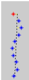
Figure 2.5 Regression line through ten node centres in one frame of a video
