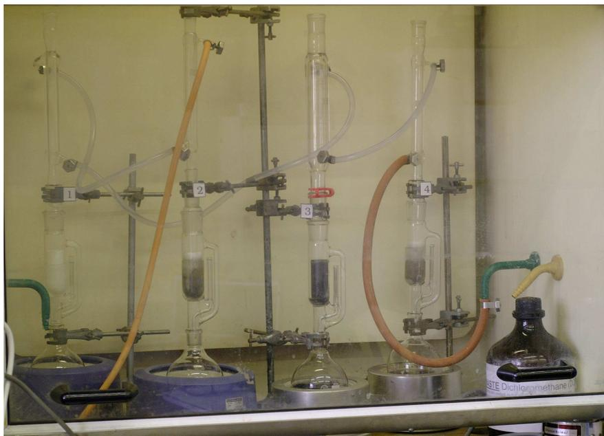
Figure 4.8: Soxhlet reflux extraction
