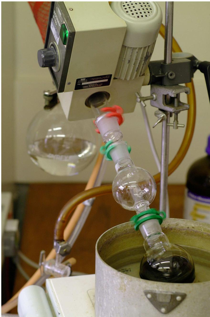
Figure 4.9: Buchi rotary evaporator
