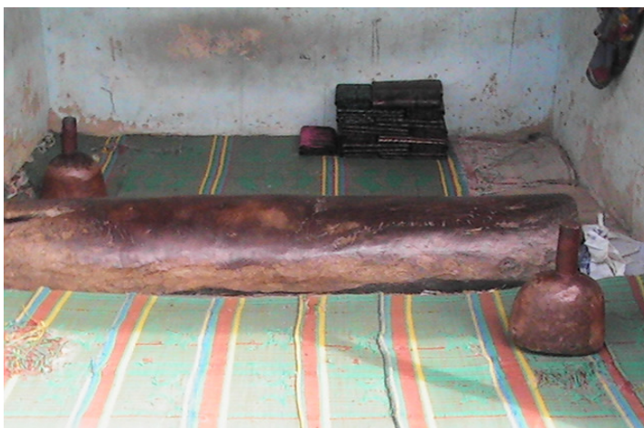
Image 15: Photograph showing wooden rod use to beat and smoothen resist dyed fabrics.
