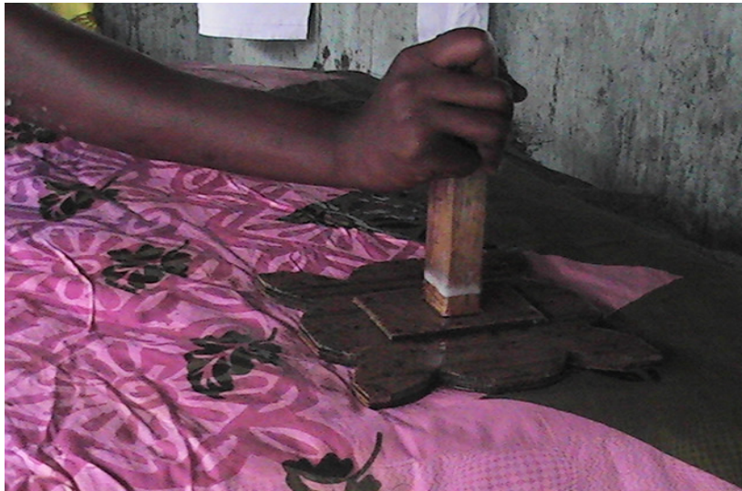
Image 12: Photograph showing transfer of wax design on fabric using wooden block
