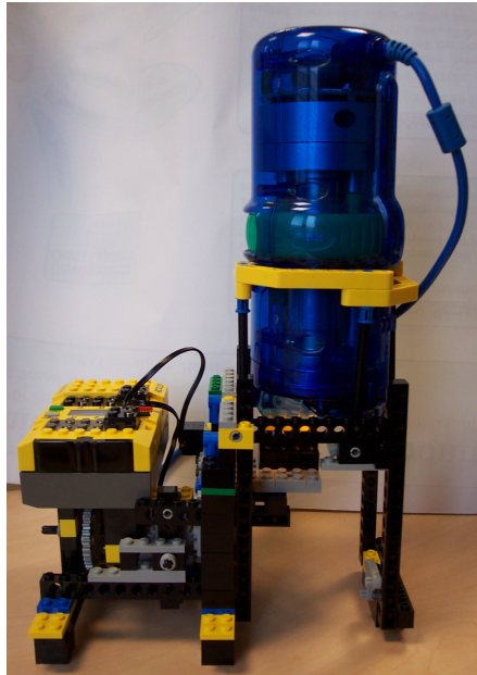
FIGURE 6.1: The IntelPlay microscope mounted in the LEGO frame.
