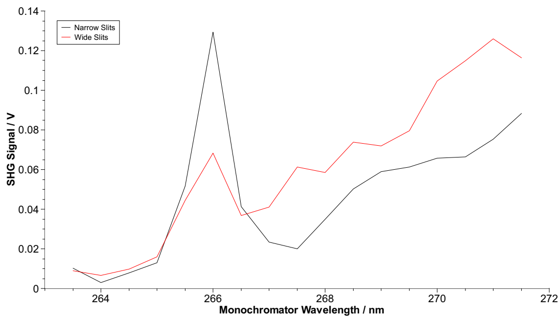
FIGURE 9.7: Monochromator scans for 10^{-5} \text{ mol dm}^{-3} R6G solution.
