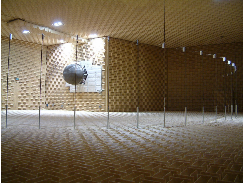
Figure 7.2: Rig including turbulence control screen (TCS) installed in the AneCom Test Facility.
