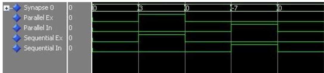
Figure 4-13: Single Input Threshold Block Simulation
