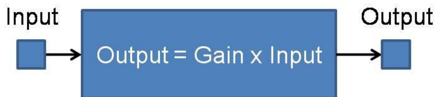
Figure 3-9: Signal Flow Model Example
