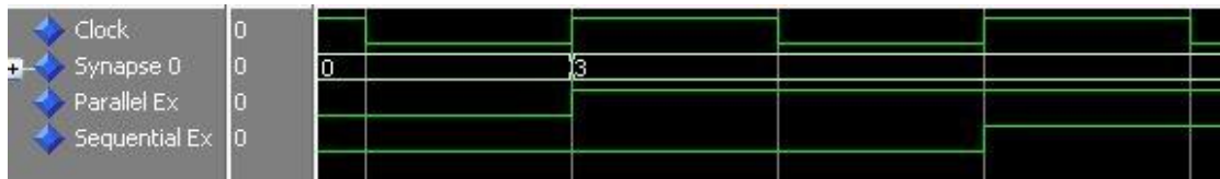
Figure 4-14: Single input simulation showing the signal lag
