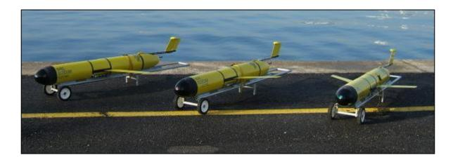
Figure 2.6 – A picture of three slocum gliders from the Webb Corporation [55] where the horizontal wings are the lift surfaces that enable forward motion.
