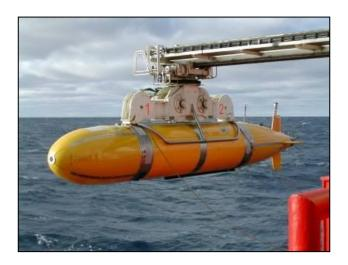
Figure 2.4 – Picture of the AutoSub being deployed in the ocean from a scientific vessel [courtesy of the National Oceanographic Centre, Southampton].
