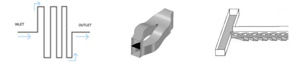
Figure 2.22*a*,  $b \, c \sim c$  – Illustrations of the channel shapes for the three main micromixer categories *a*) serpentine or chicane mixer, *b*) split and recombine [151] and *c*) herringbone or grooved channel [152].
