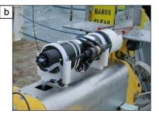
Figure 2.20a  $c^{\infty}b - a$ ) S.U.V.6 detection system mounted on a rosette frame and b) I.S.U.S. mounted on a Chelsea technologies Seasoar.
