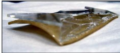
Figure 3.8 – Picture of a glass, epoxy and treated P.T.F.E. construct that has shattered during cooling.
