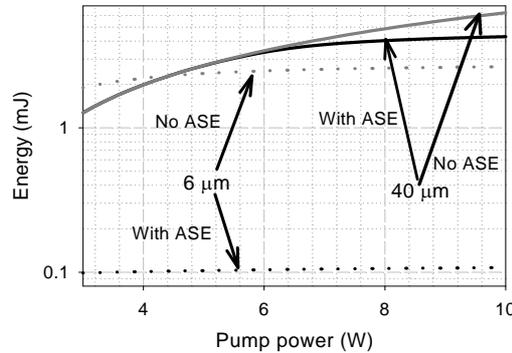
Fig. 1. Maximum extractable energy versus pump power for different core sizes.
