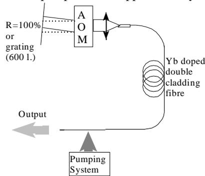
Fig. 2 Experimental setup
