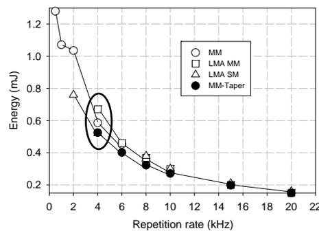
Fig. 3 Pulse energy versus repetition rate.
