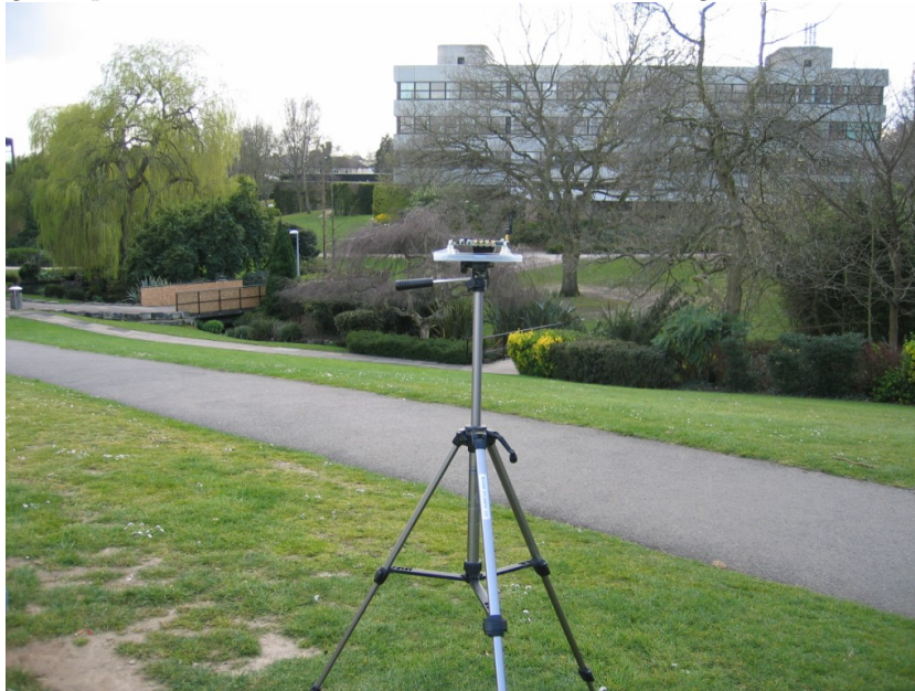
FIGURE 4.19: Photo showing NLOS test location on University of Southampton campus. Initiator placed on tripod stand and interfaced to laptop computer for data extraction and logging. Responder moved around park area with obstructed and unobstructed signal path. March 2007.
