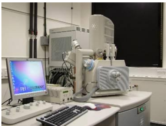
FIGURE AP 5.1 : The environmental scanning electron microscope at the Centre for Advanced Microscopy at the University of Reading [368]
