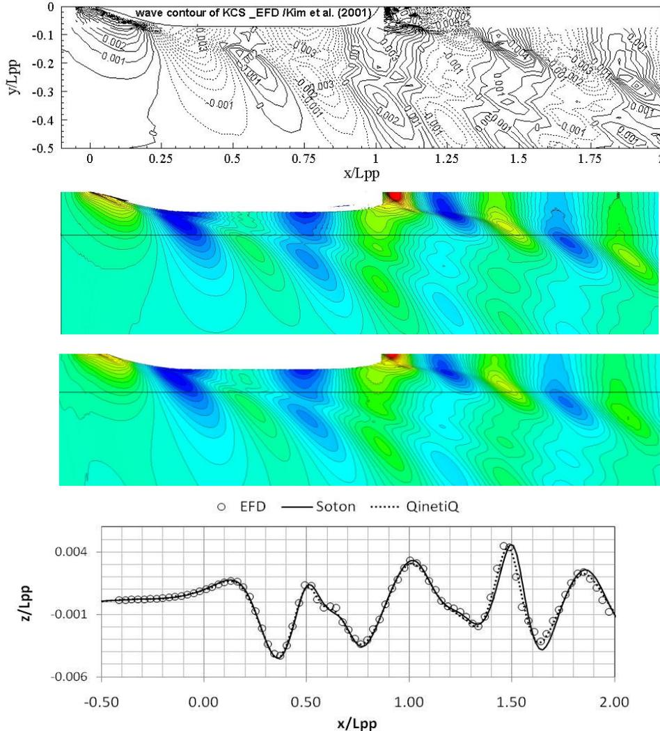
Fig.6 Free surface elevation,  $z/L_{pp}$ , of global wave pattern, at  $Fn=0.26$ , for (Top Down) Experimental data, SOTON CFD results and QinetiQ CFD results. Contours range from  $z/L_{pp} = -0.005$  to  $0.010$  in steps of  $0.0005$ . The straight lines represent the positions of the wave cut at  $y/L_{pp} = 0.15$  which are plotted against EFD data for both meshes (Bottom).
