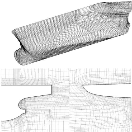
Fig.3 QINETIQ: Hull surface mesh structure (top), O-grid structure at stem from the side (left) and from the stern (right), for the coarsest mesh containing 1M elements.
