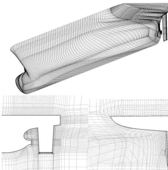
Fig.4 QINETIQ: Hull with rudder surface mesh structure (top), O-grid structure at stem from the side (left) and from the stern (right), for the coarse mesh containing 1M elements.
