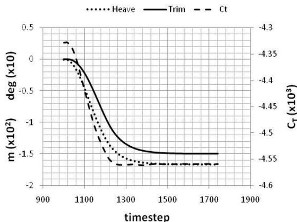
Fig.8 Example time history of a sinkage and trim simulation for  $F_n = 0.2816$  using the finest mesh (9M).
