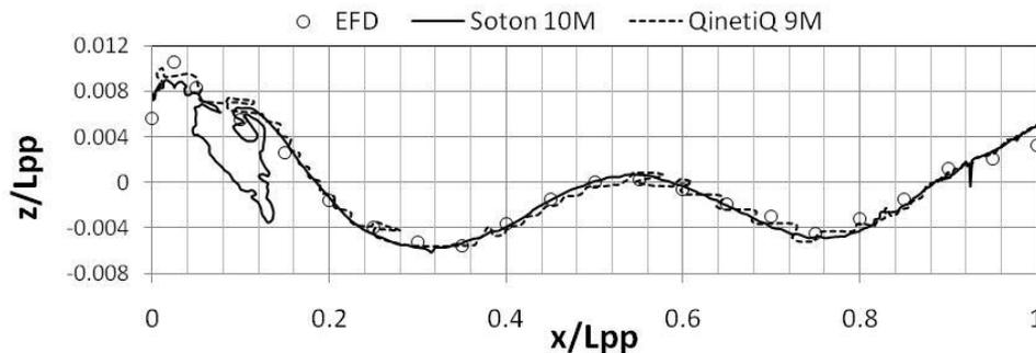
Fig.7 Comparison of free surface elevation along the surface of the hull plotted against EFD data at  $Fn=0.26$ .
