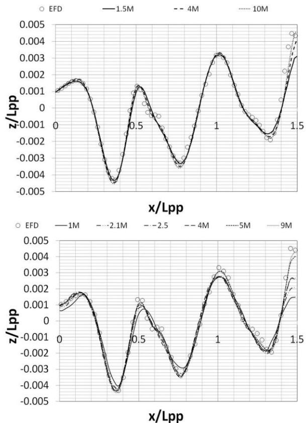
Fig.5 Comparison between experimental (EFD) and CFD wave elevation at a distance of  $y/Lpp=0.15$  from the ship centreline at  $Fn=0.26$ . Southampton results (top), QinetiQ results (bottom). The Forward perpendicular is positioned at  $x/Lpp=0$ .
