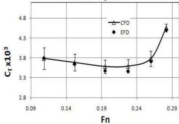
Fig.9 Comparison of EFD and CFD variation of total resistance with Froude number, with numerical uncertainty error bars.
