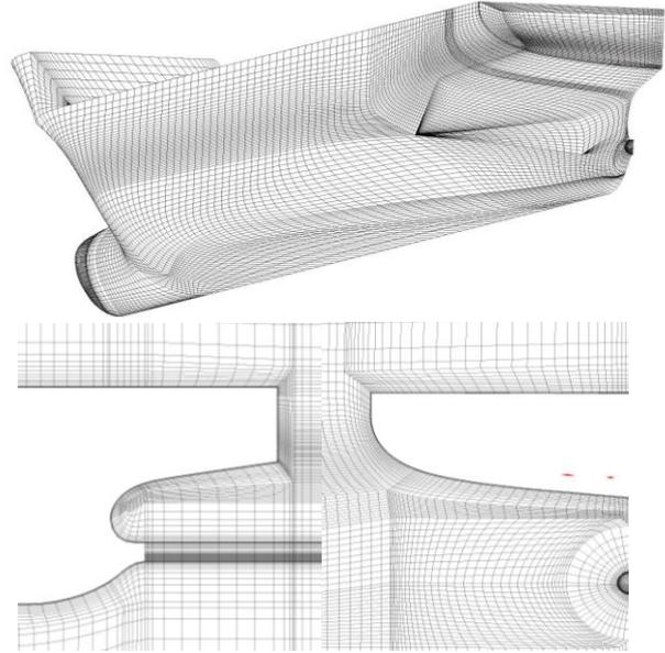
Fig.2 SOTON: Hull surface mesh structure (top), O-grid structure at stern from the side (left) and from the stern (right), for the initial mesh containing 0.8M elements.
