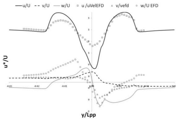
Fig.10 Velocity components down stream of propeller ( $x/L_{pp}=0.911, z/L_{pp}=-0.03$ )
