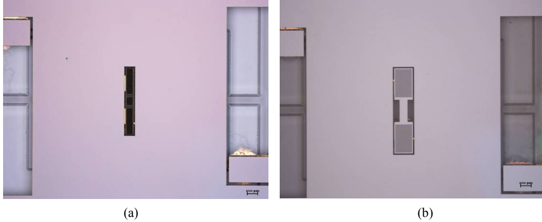
Figure 5.15: Micrograph of success DRIE etch showing that the silicon layer under the photoresist mask was not etched on the Silicon/Pyrex stack for the (a) RF MEMS switch design (b) a RF MEMS switch with a different armature design.
