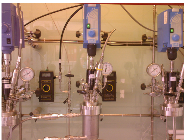
Figure 2.19: Steel autoclave for high-pressure (40 bar) catalytic tests.
