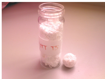
Figure 2.17: Spherical ball formed in the polymerisation of ethylene in experiment C4 (see table 12.1 for conditions).
