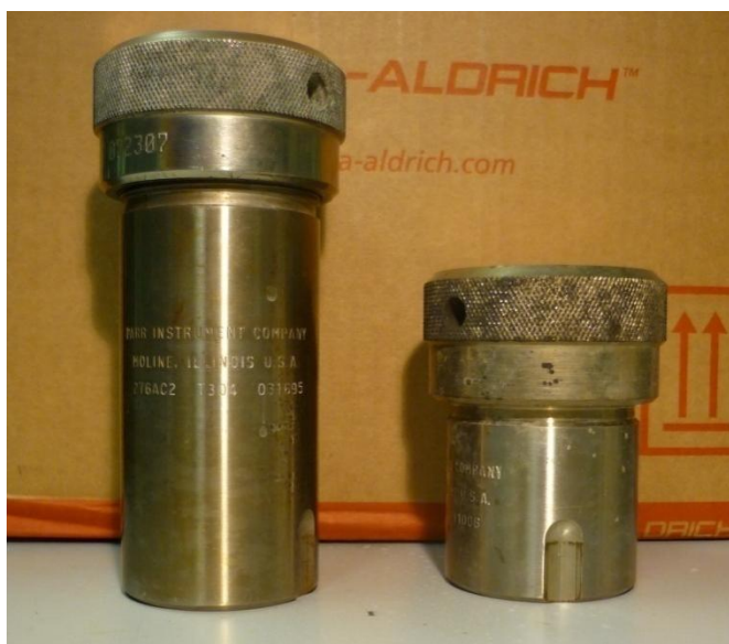
Figure 2.1: Image of Teflon-lined steel Parr autoclaves (23 mL on left and 45 mL on right)
