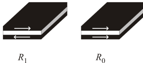
Figure 1.12 – Binary memory storage in tunnelling magnetoresistive junctions. Here, R_1 > R_0 .
