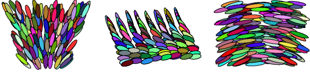
FIGURE 2.2: The three common liquid crystal disclinations, all of which have a different elastic constant. The left hand image shows the splay disclination, this has elastic constant K_1 . The middle image shows the twist disclination, this has the elastic constant K_2 . The right hand image shows the bend disclination, this has elastic constant K_3 .
