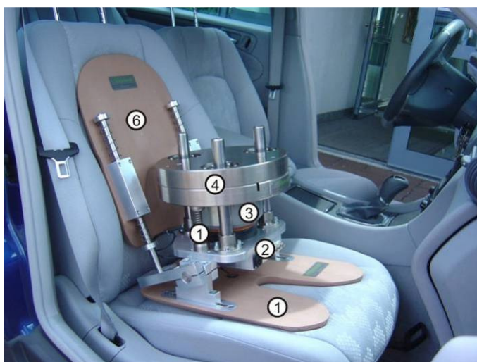
Figure 2.35 MEMOSIK active anthropodynamic dummy (from Wölfel group, 2008).
