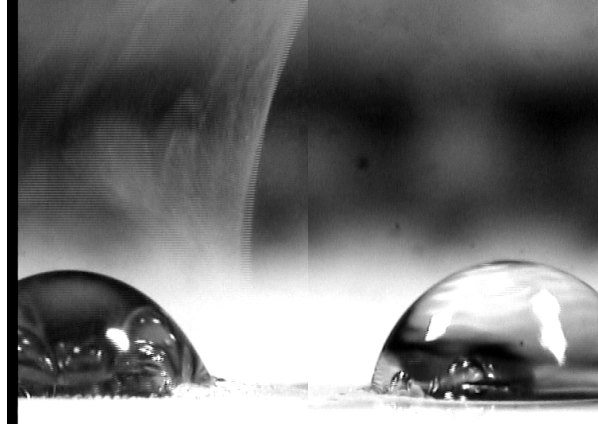
Figure 4-14 High rotating flow motion and droplet oscillation due to the application of low frequency (500 Hz). This phenomenon at high voltage (110 V) stopped droplet movement to the interdigitated region where the mixing is taking a place. With the voltage on continuously, bubbles were created inside the droplets and insulated breakdown occurred.
