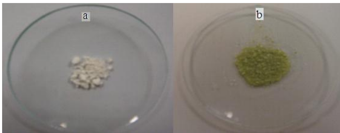
Figure 5.6 The colour testing of a) \text{MNCS}_2@\text{SiO}_2 particles before dispersion in Cu (II) solution b) \text{MNCS}_2@\text{SiO}_2 particles after dispersion in Cu (II) solution
