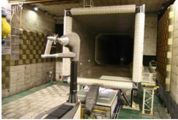
Figure 4.1: Experimental setup of Rolls-Royce's RIG145 in DNW, Netherlands.
