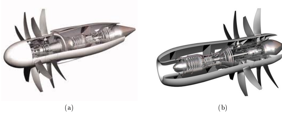
Figure 1.1: Contra-rotating open rotors in (a) puller and (b) pusher configuration. Credits Rolls-Royce.
