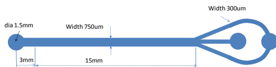
Figure 2 Planar separator design showing channel arrangement
