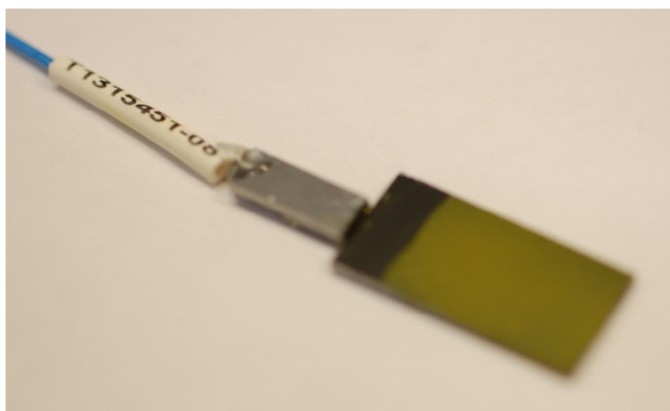
Fig. 6.15 The Bragg device spray-coated with a thick film of the azobenzene functionalised silicone polymer, 7. The first 4 mm were left uncovered to leave a reference Bragg grating.
