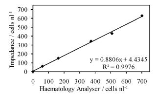
**Fig. 7** Platelet data from clinically sourced, diluted human whole blood samples, showing excellent linearity between the absolute platelet counts obtained from the impedance cytometry system and the hospital central lab haematology analyzer.
