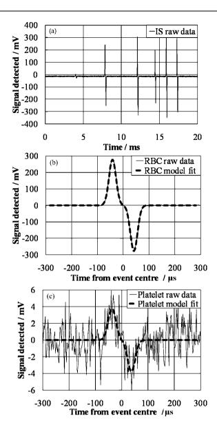
Fig. 4 (a) Time trace of the unprocessed data captured by the impedance system. The voltage signal is the magnitude of the impedance measured at a single frequency. (b) Voltage from a single red blood cell (RBC) ( $\sim$ 70  $\mu$ m³) event. The raw data and fitted data are shown. (c) Similar signal for a small ( $\sim$ 1  $\mu$ m³) platelet, with the raw data and fitted model.
