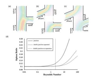
Fig. 3 Simulations of flow profiles in microfluidic junction of different designs at Re = 2.2. (a) Single T junction. (b) Separated double junction. (c) Optimally spaced double junction. (d) Siphon ratio as function of Reynolds number for the different designs.
