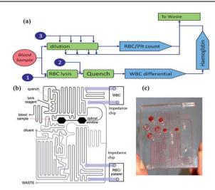
**Fig. 2** (a) Diagram of the WBC/RBC chip processes incorporating lysis and quench of the blood, followed by WBC count (with optical windows for haemoglobin). Dilution of the blood for RBC/PLT analysis is shown in the upper arm. (b) CAD drawing of the microfluidic block showing the different length channels, the input ports and the two impedance chips. (c) Photograph of the final microfluidic device made in PMMA.
