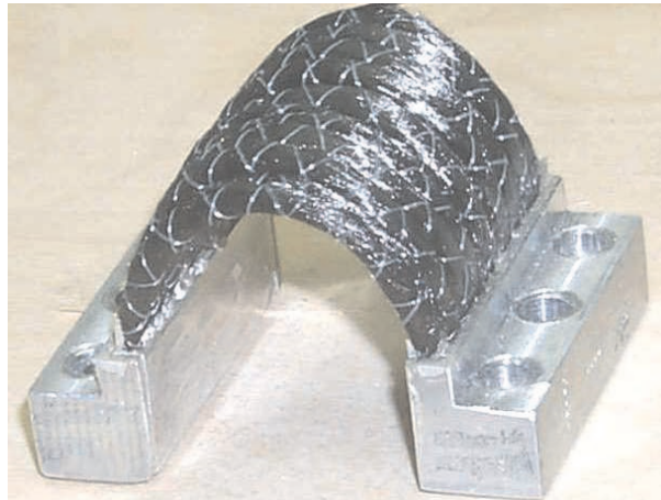
Figure 9.13: An example of a thermal strap, ©Technology Applications, Inc.
