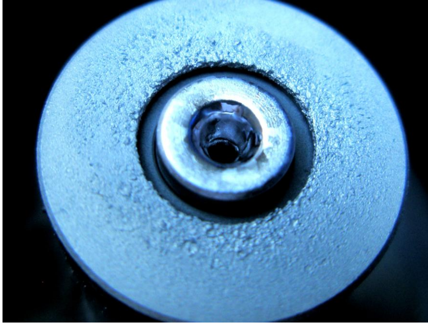
Figure 136 T6 discharge cathode tip post test image
