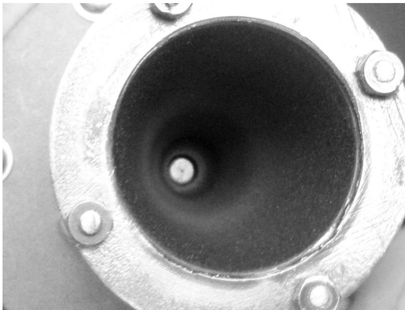
Figure 127 Image showing post test analysis of the T5CA anode with distinctive regions of arc attachment.
