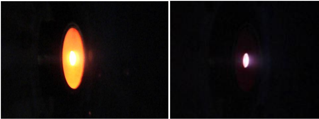
Figure 67 T5FO during operation with argon at 70.3W (3.2A) at 21V with 0.05\text{mgs}^{-1} (left) and 12.8W (0.8A) at 15V with 0.8\text{mgs}^{-1} (right)
