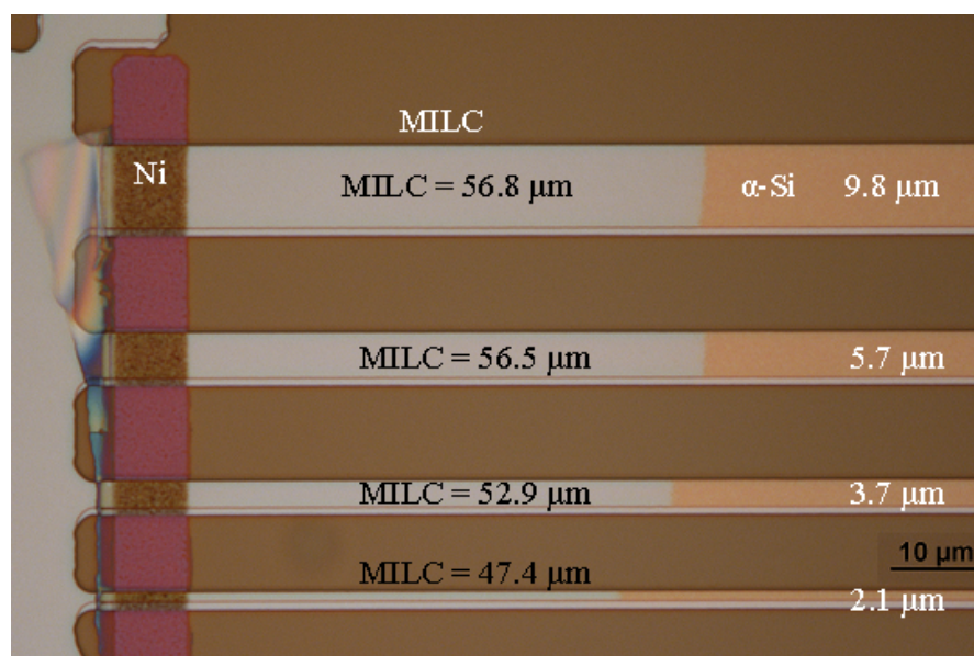
FIGURE 5.13: Nomarski micrograph of lateral crystallisation on LPCVD \alpha -Si ribbons of different widths on oxide after a 550°C anneal for 10 hours. No delineation etch was given to the sample.
