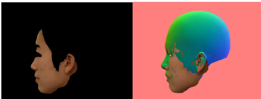
FIGURE 4.10: Image of least squared rigid registration of base mesh to feature points
