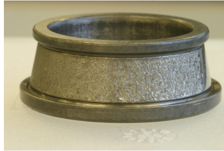
Figure E.7 Photographic evidence of inner race spallation to bearing 2.
