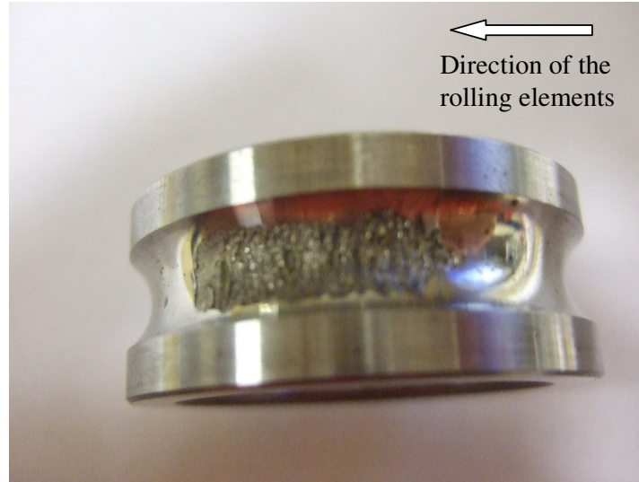
Figure 6.15 Photographic evidence of damage to bearing number 2.
