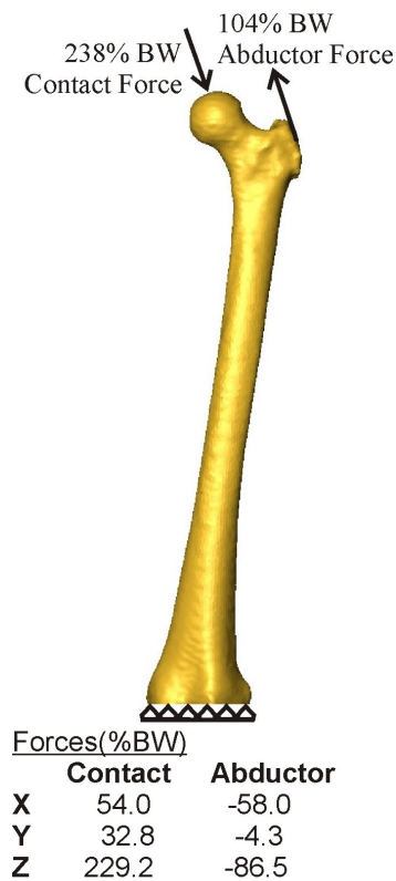
Figure 5.8: Illustration of the loading condition defines by Heller et al. [33]
