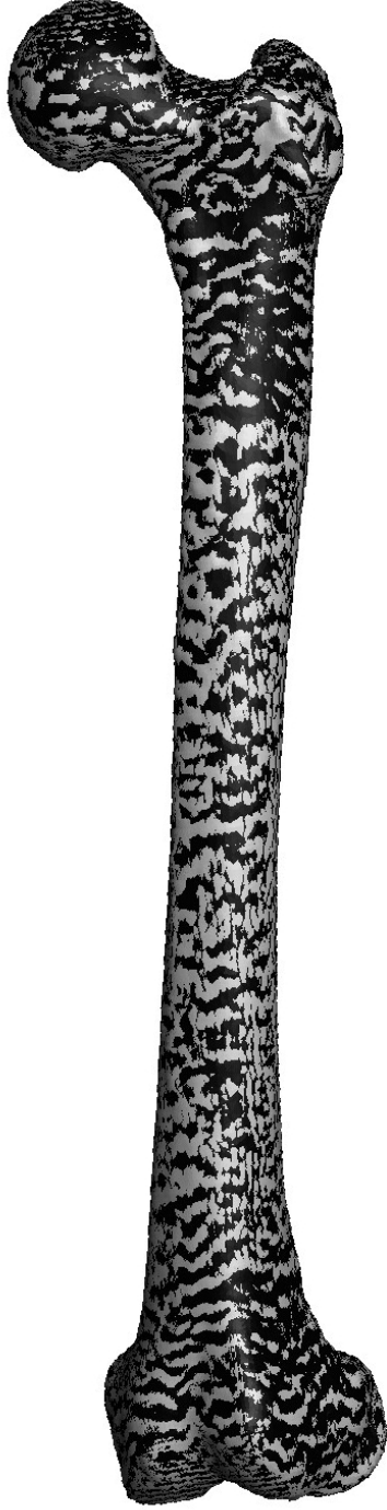
Figure 3.9: Illustration of the target mesh (black) with morphed baseline mesh (grey) superimposed, showing the accuracy achievable by the registration scheme.
