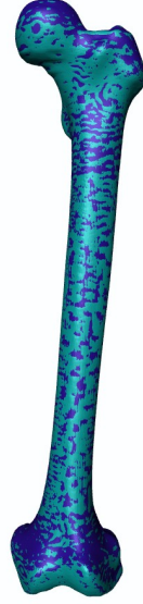
Figure A.2: Target mesh (dark) with morphed baseline mesh (light) superimposed, showing the accuracy achievable by the registration scheme
