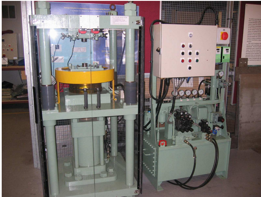
Fig 6.1: HPT facility showing the two sets: the control panel and the high pressure press.
