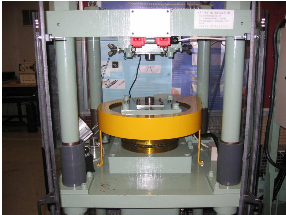
Fig 6.3: The high pressure torsion facility showing the upper and lower anvil.
