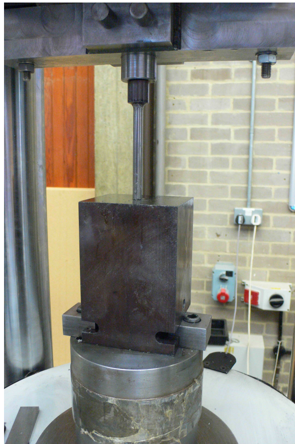
Fig. 3.1: Photographs of the experimental facility used in the ECAP experiments showing the die and the plunger.
