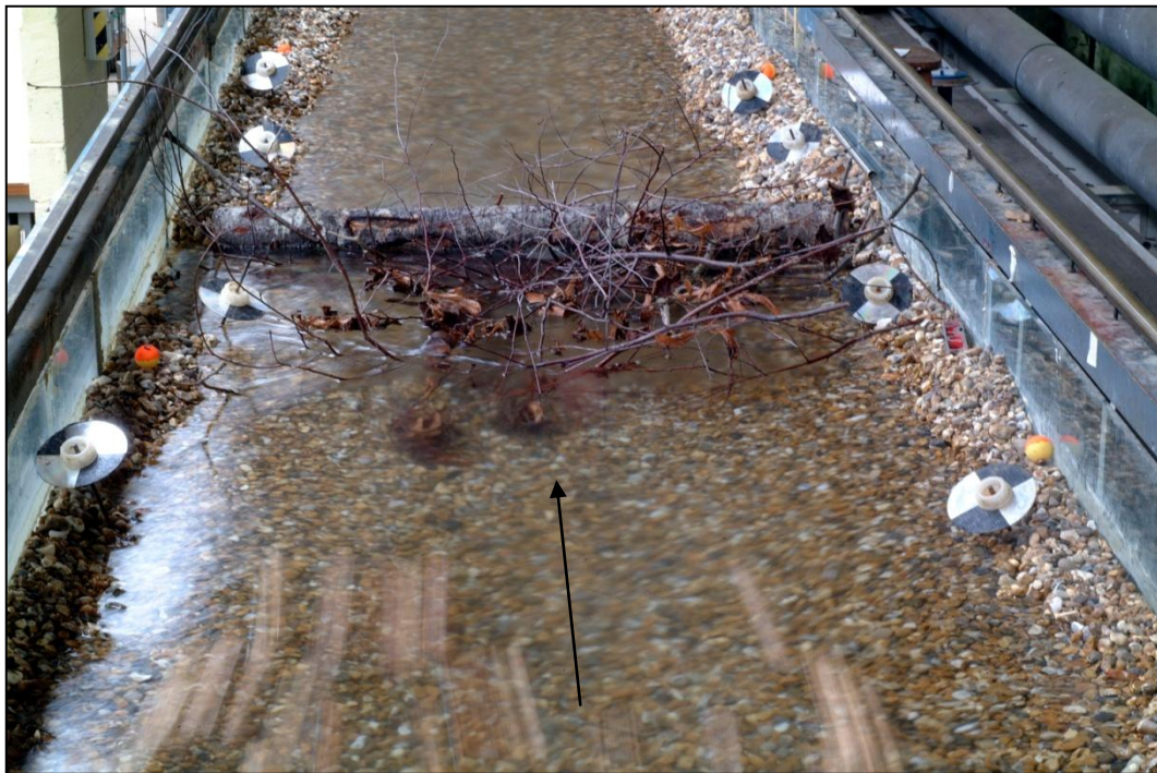
Figure 7.8.1: Large Wood Accumulation in a flume environment. The arrow shows the direction of flow.
