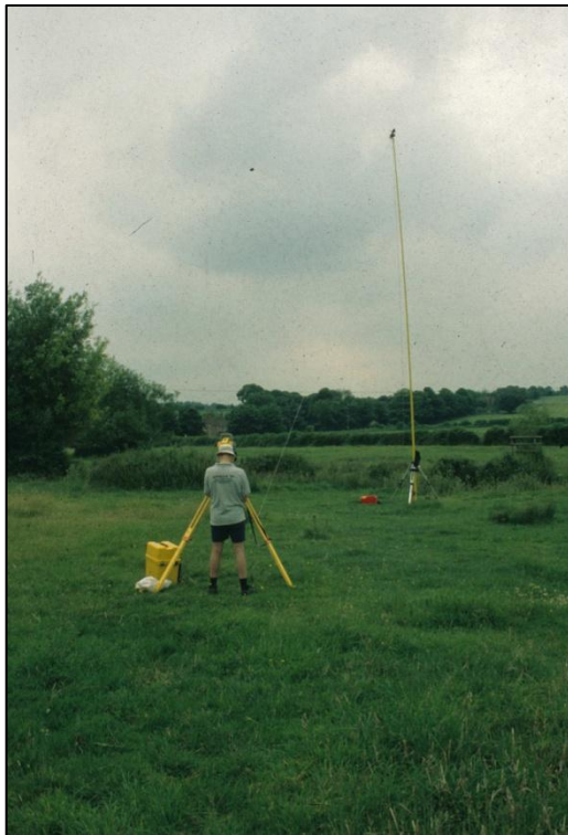
Figure 8.4.1: The Extendable Pole used for the Large Scale Particle Image Velocimetry.
