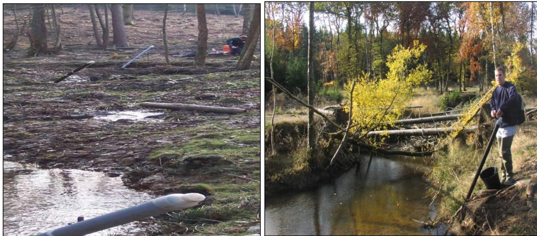
Figure 6.6.1: Two Photos of Crest Gauges used in the field to monitor peak water levels.
