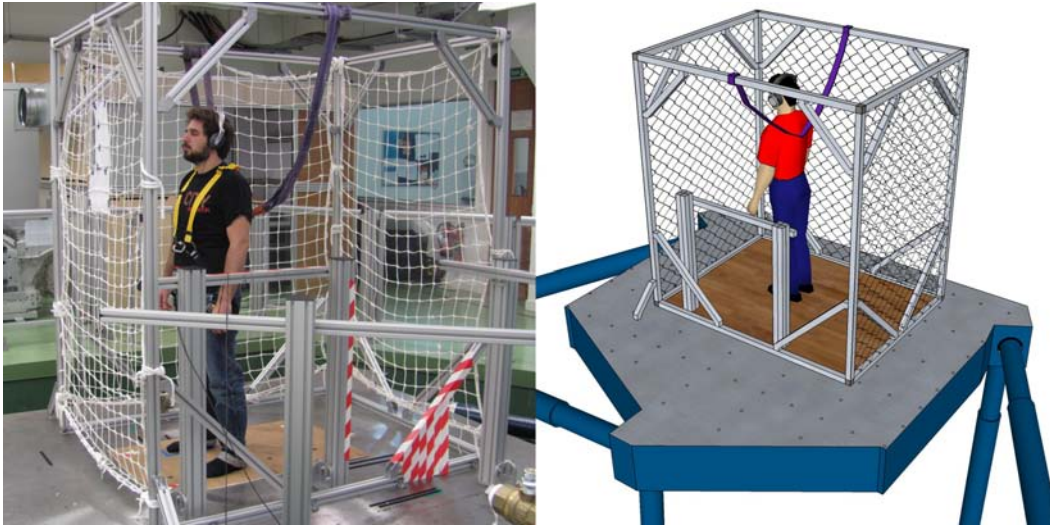
Figure 8.1: Photograph and model of the safety frame mounted on the 6-axis motion simulator.
