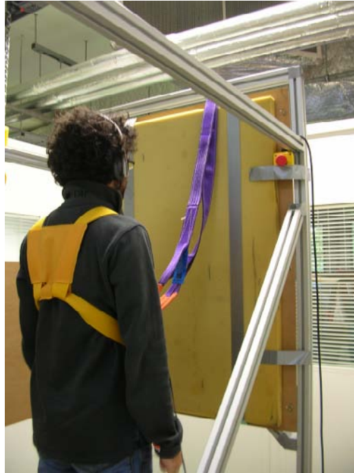
Figure 3.11: Harness system used on the single-axis vibrators (horizontal and vertical).
