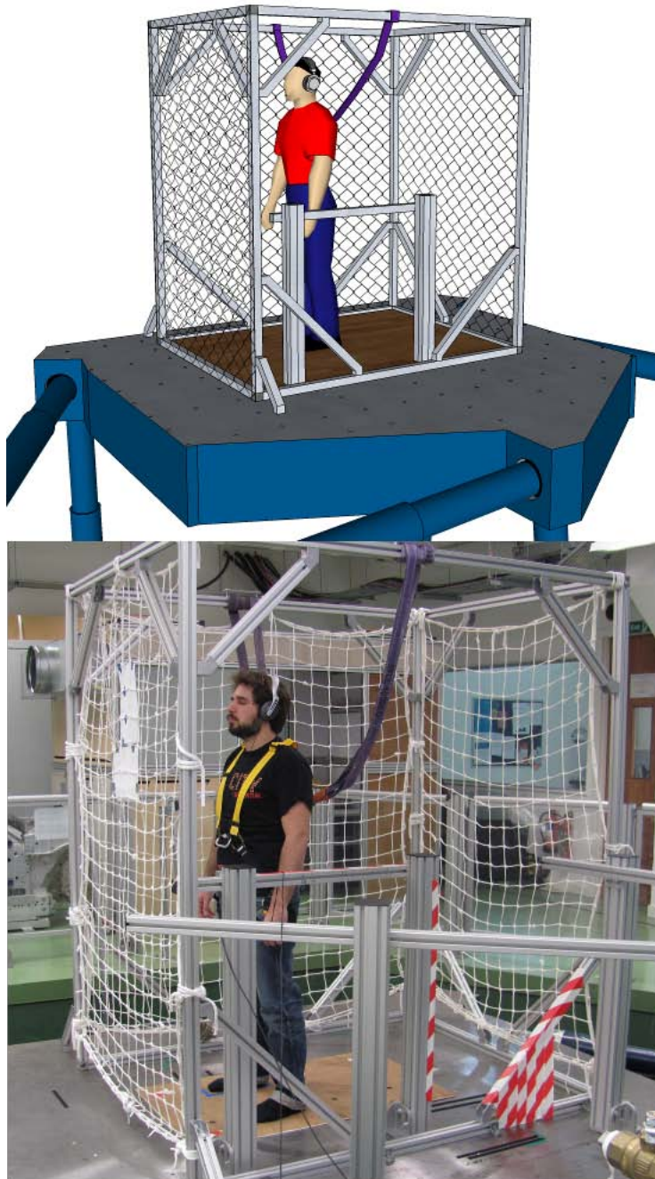
Figure 5.1: Photograph and model of the safety frame mounted on the 6-degrees-of-freedom motion simulator.
