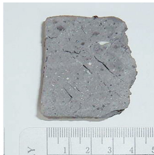
Figure 4: A raw, dried brick was cut to size to fit into a laboratory tube furnace and fired at 1050°C in inert argon gas. Shown is a slice cut off after firing.
