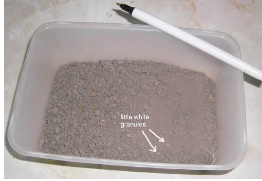
Figure 5: Dried raw material used for brickmaking. Little white grains were discernable by eye. Using X-ray diffraction, these grains were identified as a mixture of calcium sulphate hydrate CaSO_4 \frac{1}{2}H_2O and quartz.
