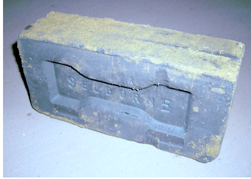
Figure 3: For elemental wavelength dispersive XRF-analysis of the clay, a dried brick was cut open and several grams of clay were taken out of the centre of the dried brick.
