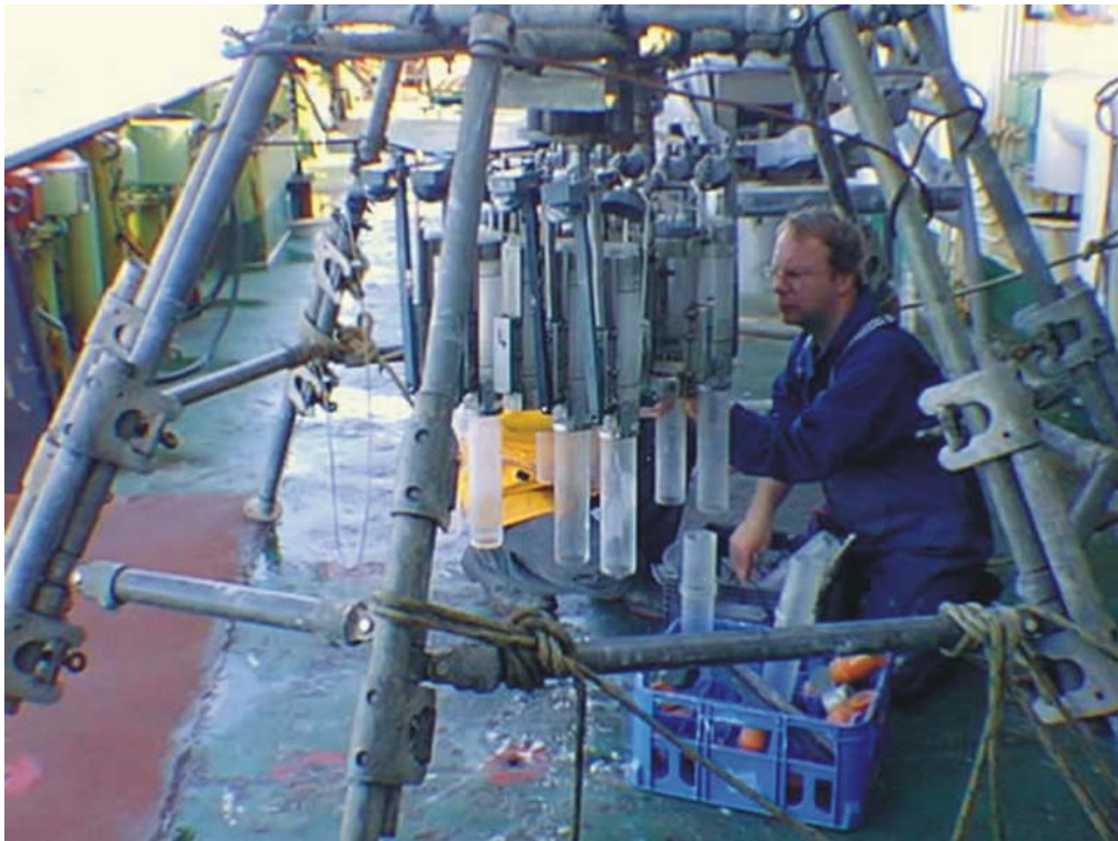
Figure 2.3. Multiple corer equipped with 57 mm diameter tubes, seen here loaded onto the coring head. Picture from Alan Hughes.
