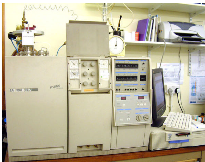
Plate 4.3: The Carlo Erba CHN analyser was used to assess the C+N content of Posidonia oceanica tissue.
