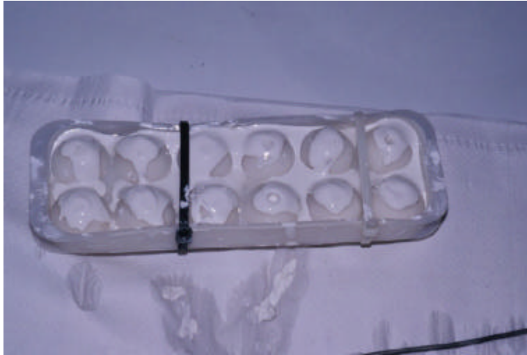
Plate 3.4: Plaster balls were prepared by inserting the plaster mixed with water into ice cube moulds.
