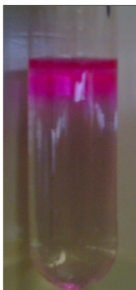
Figure 4.6. (a) Sucrose density gradient analysis. Lipid (●), KvAP (○), and KvAP pore domain only mutant (△) were run alone on separate sucrose density gradients. (b) Photograph of lipid alone after centrifugation at 80,000 g for 18 hours on the discontinuous sucrose density gradient
