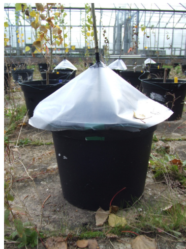
Fig. 2. Rain covers used to shield drought treatment pots from rainfall.
