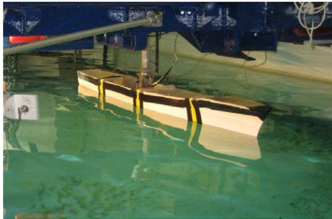
**Figure 1: The flexible model hull installed in the towing tank**
