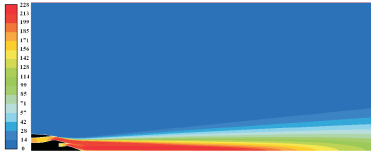
Figure 6.17 – CFD for isothermal short cowl nozzle with VR 1.0.
