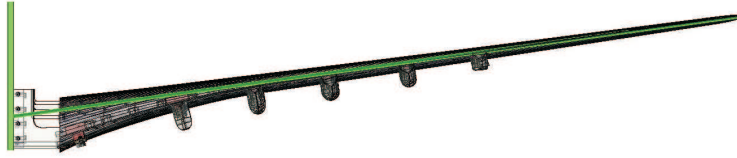
Figure 4.5 – Diagram of profile of the flat plate wing versus a realistic wing.
