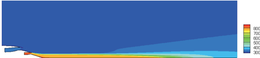
Figure 6.19 – Temperature profile from CFD for sideline jet condition with short cowl nozzle, TR=4.0 .
