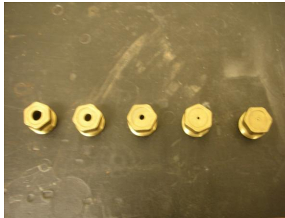
Figure 3.4. Circular leak holes of 8 mm, 6 mm, 4 mm, 2 mm, 1 mm diameter.
