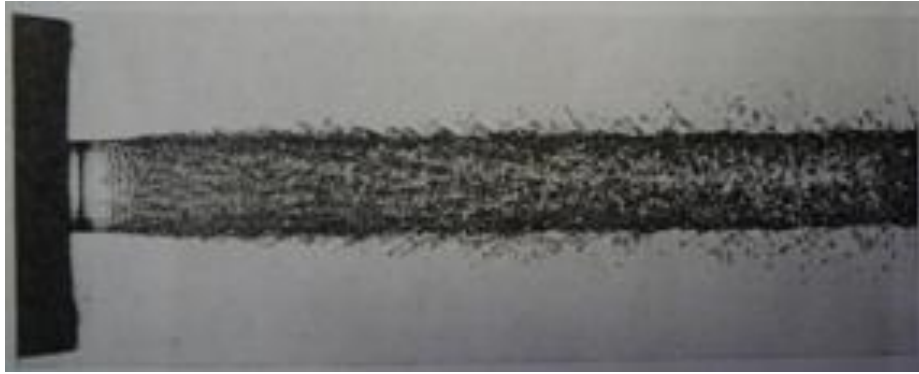
Figure 2.6. Water jet emerging from 0.635 cm diameter nozzle into stagnant air. Jet velocity=25.3 m/s [32].
