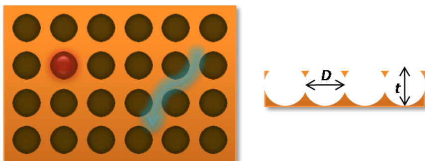
Figure 1-8 – Schematic of SSV substrate from above and side on. The Bragg plasmon is shown in blue, and the Mie plasmon in red.
