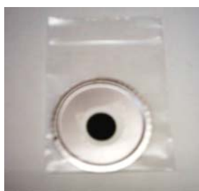
Figure 6.4 The precipitate of ^{129}\text{I} as palladium iodide ( \text{PdI}_2 ) on a filter sealed on the aluminium planchette.
