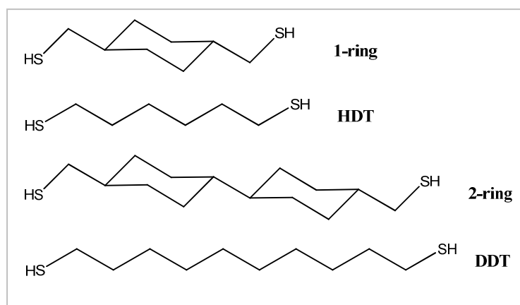
Figure 13. Insulating MWs synthesized for the STM study of the T dependence in single molecule conductivity, and their linear chain analogues (note that the free thiol is shown here but the compounds were synthesized as acetyl-protected thiols for increased stability).
