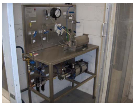
Figure 148 Autoclave for hydrogen insertion [ref 187]
