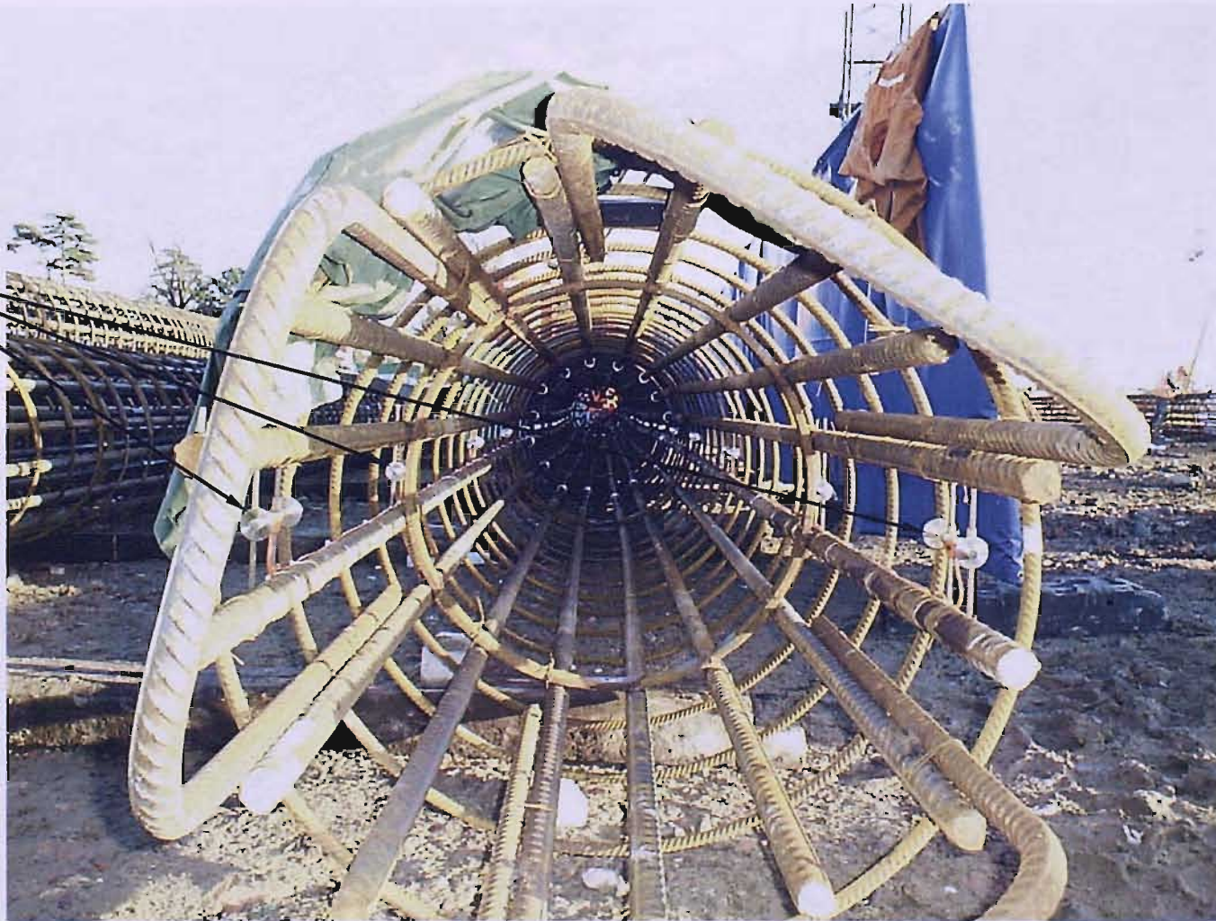
Figure 3-30: Strain gauges for measurement of pile bending moment
