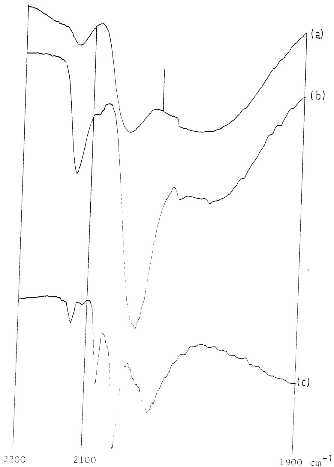
Figure 2.6. I.r. spectra ( 2\ 200 - 1\ 900\text{ cm}^{-1} ) of (a) the product from vacuum pyrolysis of (2) on \gamma\text{-Al}_2\text{O}_3 (disc), (b) the previous sample exposed for 20 minutes to 35 mm Hg of carbon monoxide, and (c) the intermediate seen from the pyrolysis of (2) on \text{SiO}_2 under carbon monoxide.
