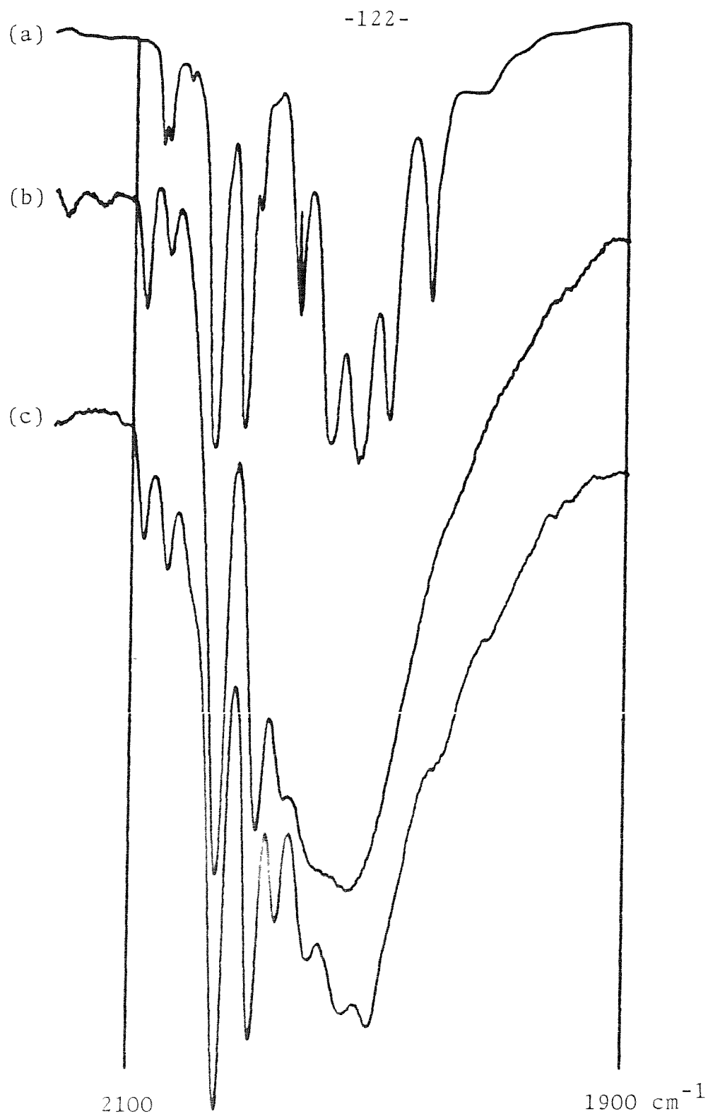
Figure 3.9. I.r. spectra of (a) an equilibrium mixture of both isomers (8) and (9) of [\text{Os}_3(\text{CO})_9(\text{H})(\text{SPr}^n)(\text{CH}_3\text{CN})] in cyclohexane, (b) a Nujol mull of the \text{CH}_3\text{CN} derivative on thiolated aerosil 380, and (c) a Nujol mull of the \text{CH}_3\text{CN} derivative on \text{SiMe}_3\text{Cl} pretreated thiolated aerosil 380.
