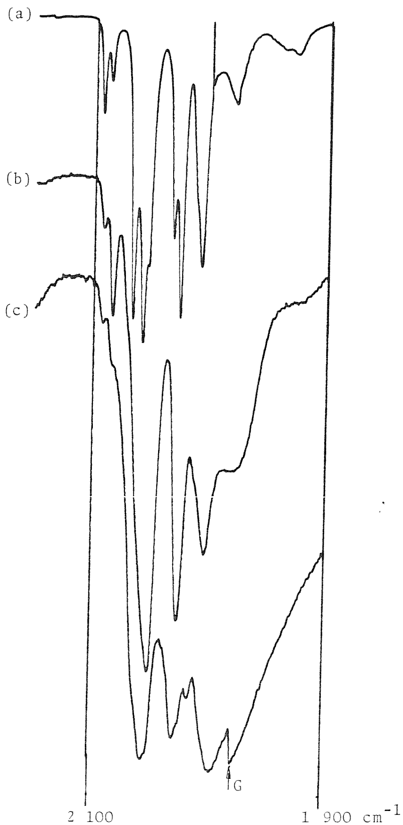
Figure 4.6. I.r. spectra of (a) [\text{H}_4\text{Ru}_4(\text{CO})_{11}\text{PPh}_2\text{Et}] in cyclohexane, (b) Nujol mull of the product from [\text{H}_4\text{Ru}_4(\text{CO})_{12}] with phosphinated silica by the photochemical method, and (c) Nujol mull of the product from [\text{H}_4\text{Ru}_4(\text{CO})_{12}] with phosphinated silica by the thermal method (G = Grating change).
