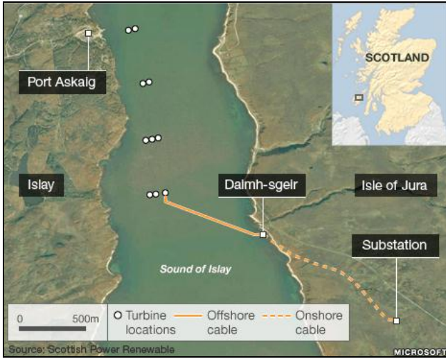
Fig. 5 Aerial view of proposed layout of Islay tidal turbine array. The streamwise and lateral separations of the devices are 20 and 1.5 diameters respectively [24]. Obtained from: http://www.bbc.co.uk/news/uk-scotland-glasgow-west-12767211 , accessed 13/05/2011.
