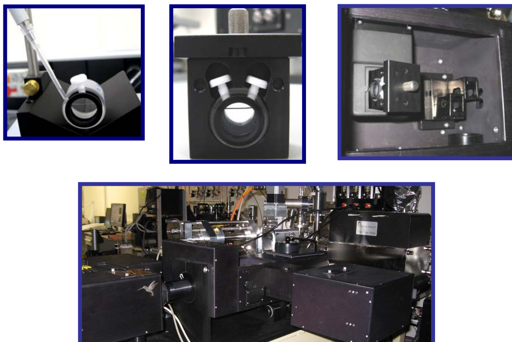
Figure 3.22: Sample in a circular cell (top) measured in Olis DSM20 CD spectrophotometer (bottom).
