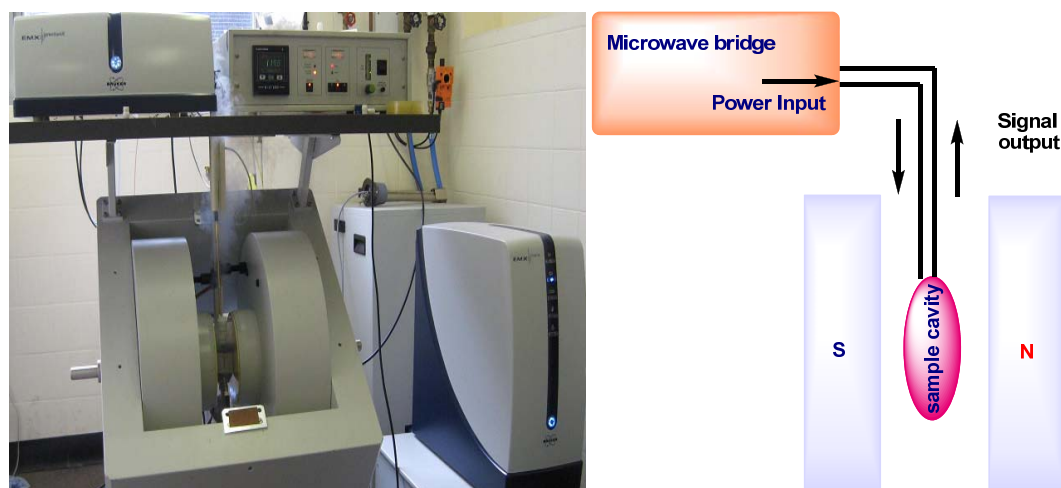
Figure 4.7: Basic components of a Bruker X-band EPR spectrometer.
